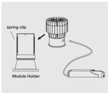
4. Attach module to module holder 5. Gently insert fixture frame & with spring clip and connect module to driver.
