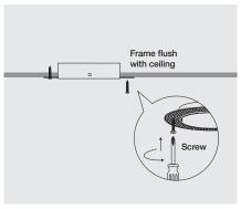
2. Secure flush mount kit onto ceiling with screws.
