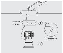
module holder from the bottom of the flush mount kit.
